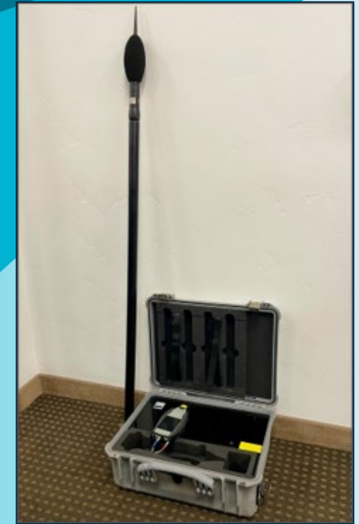
Figure 7. B&K Class I, 2250 Sound Level Meter and associated field equipment.
