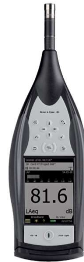
Figure 4. B&K Class I, 2250 Sound Level Meter and associated field equipment.
