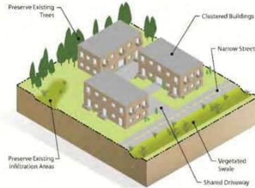
Impervious cover can be minimized by identifying the smallest possible land area that can be impacted or disturbed during site development. Reducing impervious surfaces retains the permeability of the project site, allowing natural processes to filter and reduce sources of pollution.
