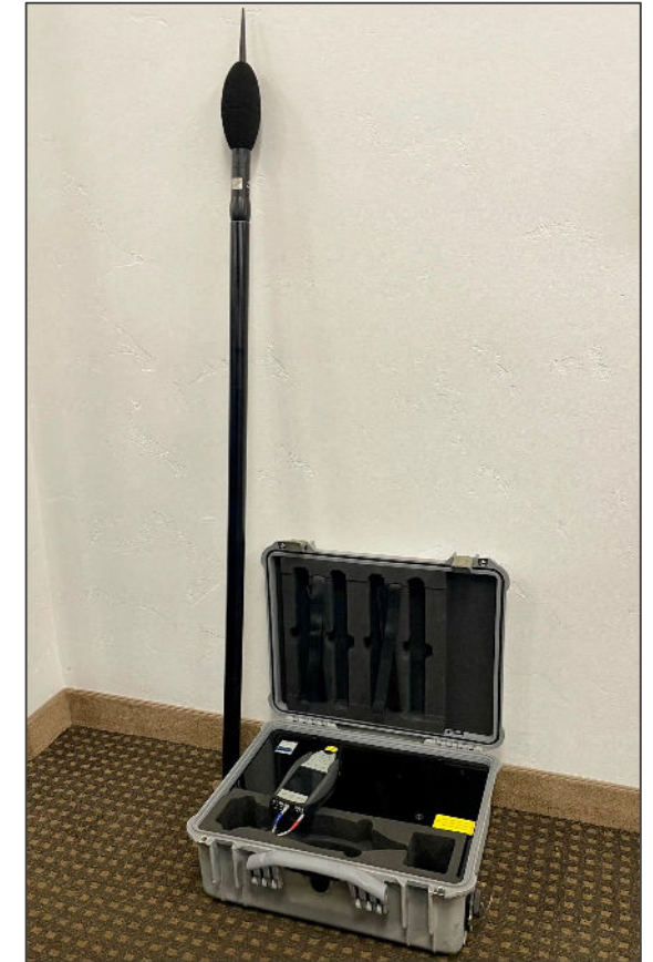
Figure 3. B&K Class I, 2250 Sound Level Meter and associated field equipment.
