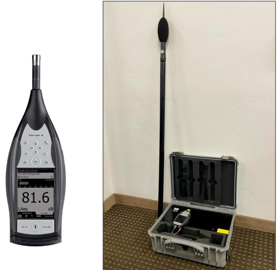
Figure 4. B&K Class I, 2250 Sound Level Meter and associated field equipment.
