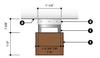
S3C.12 - Square Identification Sign - Ceiling Mounted S4C.12 - Rectangular Identification Sign - Ceiling Mounted with M3 - Mounting Bracket
