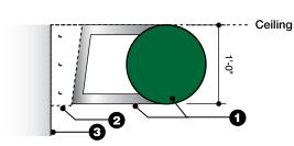
S1.12 - Circular Identification Sign with M1 - Mounting Bracket Scale: 3/4" = 1'-0"
