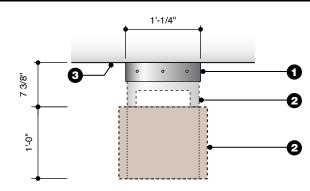
M3 - Mounting Bracket with S3C.12 - Square Identification Sign S4C.12 - Rectangular Identification Sign
