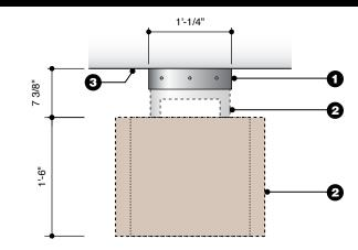
M3 - Mounting Bracket with S3C.18 - Square Identification Sign S4C.18 - Rectangular Identification Sign
