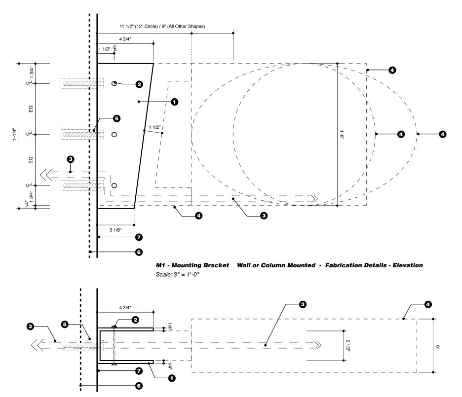
**M1 - Mounting Bracket** Wall or Column Mounted - Fabrication Details - Plan View Scale: 3" = 1'-0"
