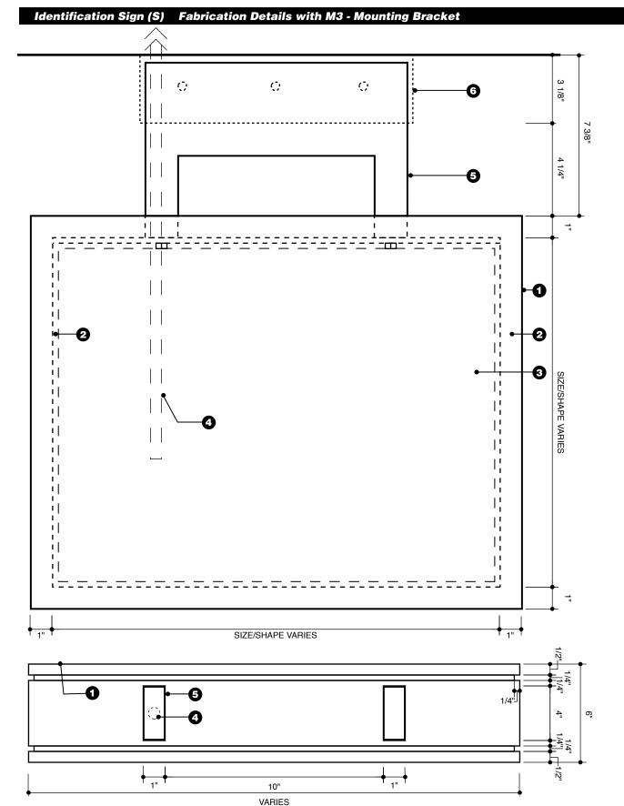
Identification Sign Fabrication Details S1C, S2C, S3C, S4C with 12", 18" Sign Faces Front Elevation with M3 - Mounting Bracket Ceiling Mounted
