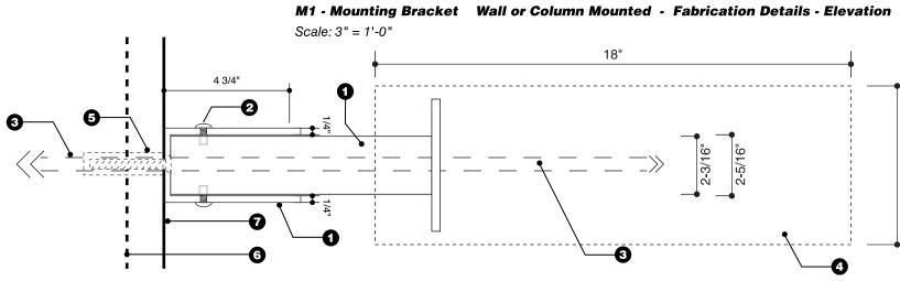
M1 - Mounting Bracket Wall or Column Mounted - Fabrication Details - Plan View
