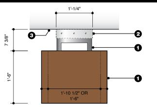
S1C.18 - Circular Identification Sign - Ceiling Mounted with M3 - Mounting Bracket Scale: 3/4" = 1'-0"
