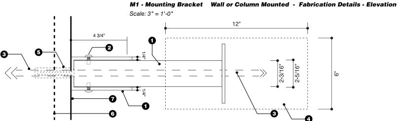
M1 - Mounting Bracket Wall or Column Mounted - Fabrication Details - Plan View
