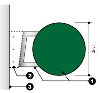
S1.18 - Circular Identification Sign with M1 - Mounting Bracket Scale: 3/4" = 1'-0"
