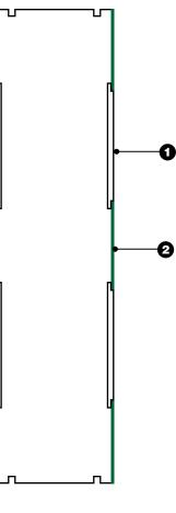
Identification Sign (S) Sign Face Fabrication - Option 2 Push-through with flush face Scale: 3" = 1'-0"
