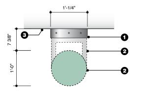
**M3 - Mounting Bracket with S1C.12 - Circular Identification Sign** *Scale: 3/4" = 1'-0"*
