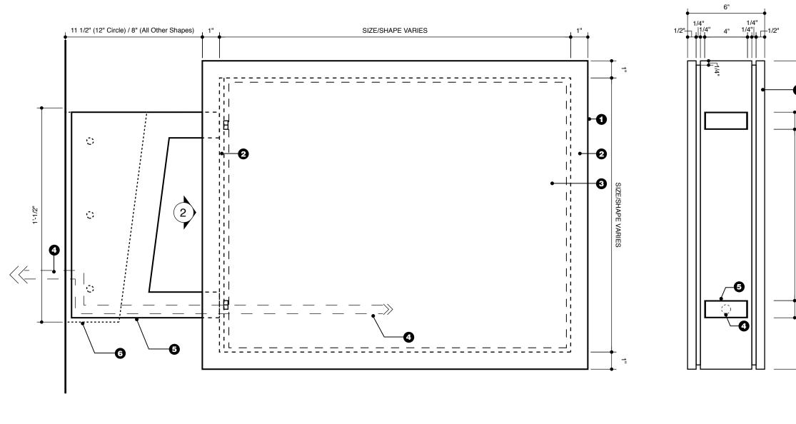
**Identification Sign Fabrication Details** Front Elevation shown with S4 Sign Face with M1 - Mounting Bracket Wall or Column Mounted
