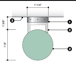
**M3 - Mounting Bracket with S1C.18 - Circular Identification Sign** Scale: 3/4" = 1'-0"
