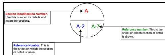
Figure 7.4.o.: Section/Detail Identification
