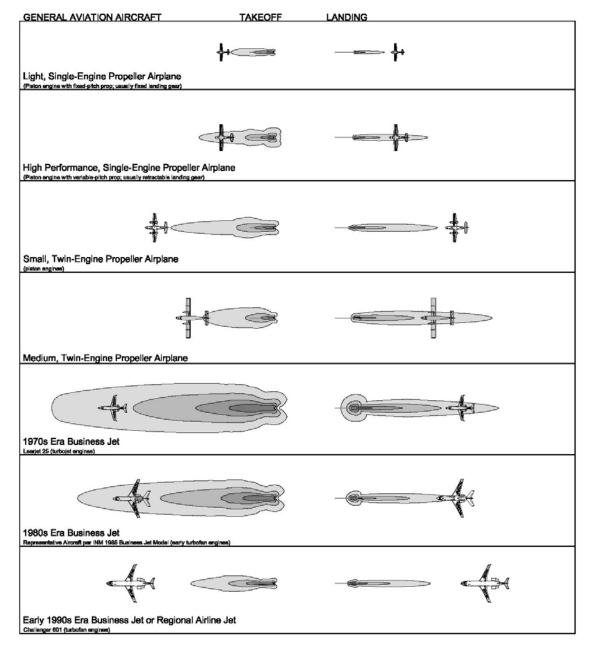
Notes: This drawing shows the relative noise levels produced by different types of aircraft during landing and takeoff. The contours represent the momentary maximum sound level experienced on the ground as the aircraft flies over. The outermost contour for each aircraft indicates a 65 dBA sound level. Additional contours are at 10 dBA increments (75, 85, and in most cases 95 dBA). Aircraft are not to scale.
