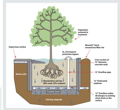
Figure 6-6. Stormwater tree pit schematic.
