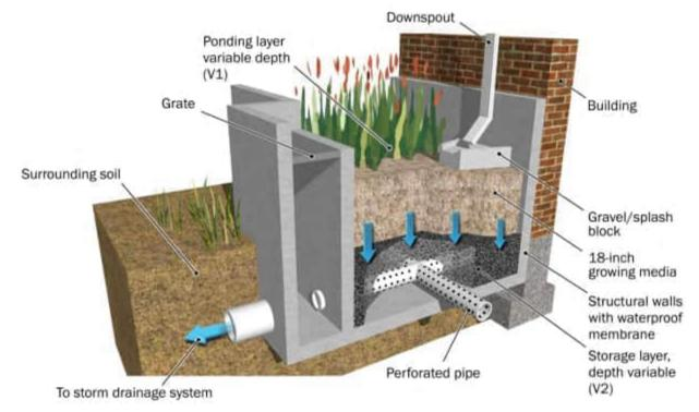
Biofiltration with impermeable liner BMP Example Illustration
