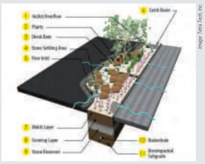
Figure 6-4. Components of a stormwater curb extension.
