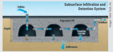
Figure 6-9. Subsurface infiltration and detention system schematic.
