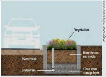
Figure 6-5. Stormwater planters, unit plan view (left) and cross section (right).
