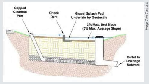
Figure 6-2. Cross-section of a bioswale designed with a check dam to control slope.
