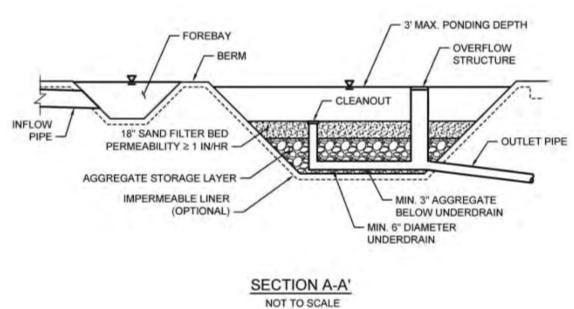
Typical Plan and Section View of a Sand Filter BMP
