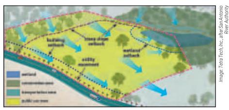
**Figure 3-2.** A base map indicates landscape and hydrologic features, necessary setbacks, existing easements and other components.
