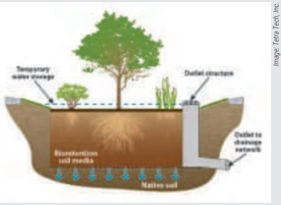
Figure 6-1. Cross-section of a common bioretention practice design.
