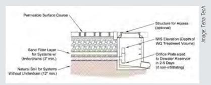
Figure 6-11. Permeable interlocking concrete pavement cross-section.
