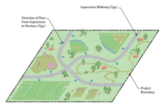
FIGURE 5-4. Self-retaining DMA Site
