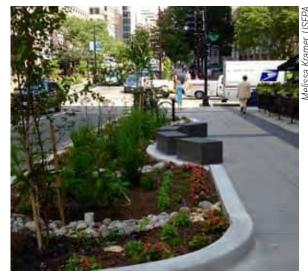
**Figure 4-36.** Seating adjacent to a bioretention unit provides an amenity for passersby and also serves as a barrier in Washington, DC.
