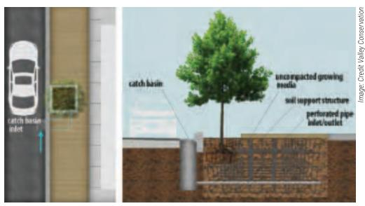
Figure 6-7. Cross section of tree box with a structural support system under the sidewalk.
