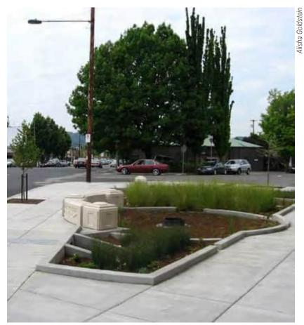
Decorative stone benches installed at the edge of a bioretention area offers a resting spot for pedestrians along Sandy Boulevard in Portland, OR.
