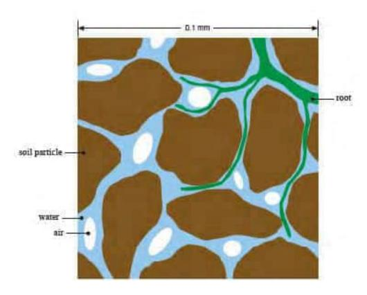
Figure G.1-3. Unsaturated Soil Composition
