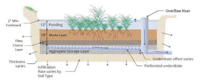
Biofiltration with Partial Retention BMP Example Illustration
