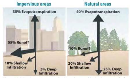
**Figure 1-1.** When impervious areas (roads, rooftops, parking lots) cover much of the land (left image), more than half the rainfall runs off and flows directly into surface waters, allowing only 15 percent of rain water to soak into the ground. In contrast, areas that are designed to mimic natural areas (right image) allow only 10 percent of rain to run off and nearly half to soak into the ground.
