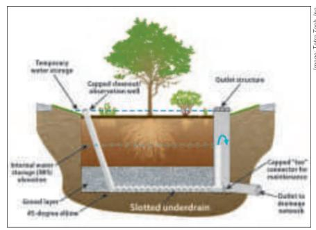
**Figure 4-25.** In this underdrain design cross-section image, an upturned pipe connected to a slotted underdrain ensures that a permanent internal water storage layer is maintained within the practice before the excess infiltrated water spills into a secondary drainage network. In this design, a surface overflow drain is included to provide added protection against high volume flows.
