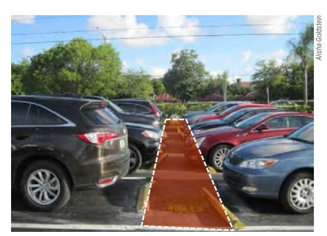
**Figure 2-13.** In this parking lot the impervious median space between facing parking stalls could be retrofitted to infiltrate runoff.
