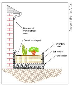
A stormwater planter can be designed to capture and treat roof runoff.
