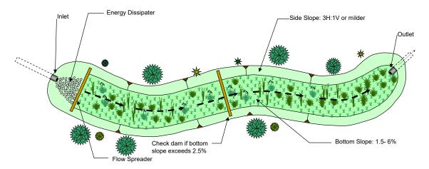
FIGURE 5-10. Schematic of a Vegetated Swale
