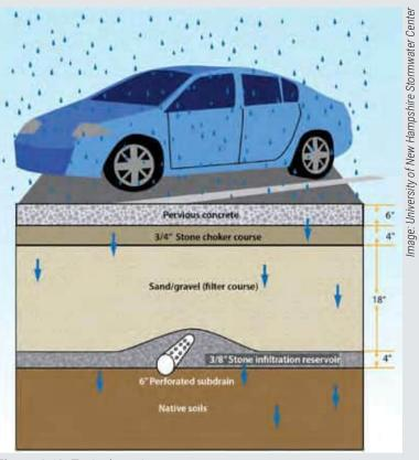
Figure 6-10. Typical pervious concrete pavement cross-section.
