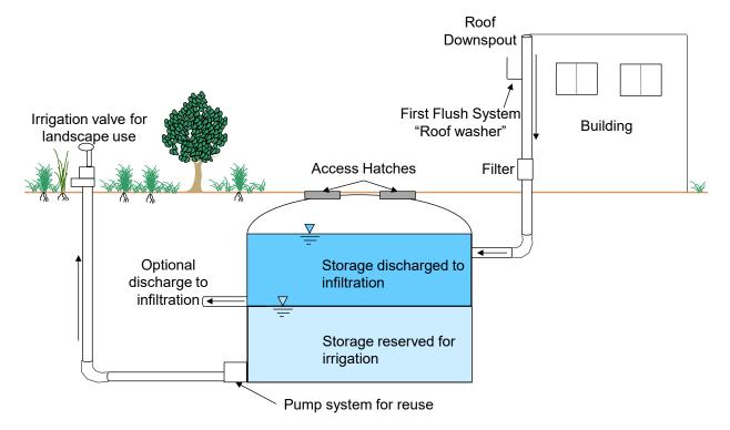
FIGURE 5-6. Schematic of a Typical Cistern
