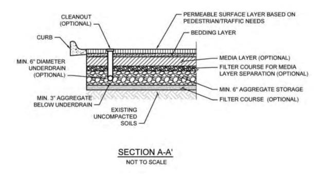
Typical Plan and Section View of a Permeable Pavement BMP
