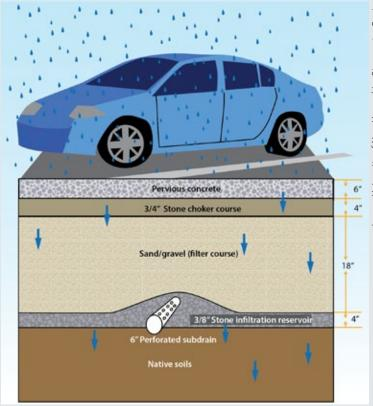
Figure 6-10. Typical pervious concrete pavement cross- section.
