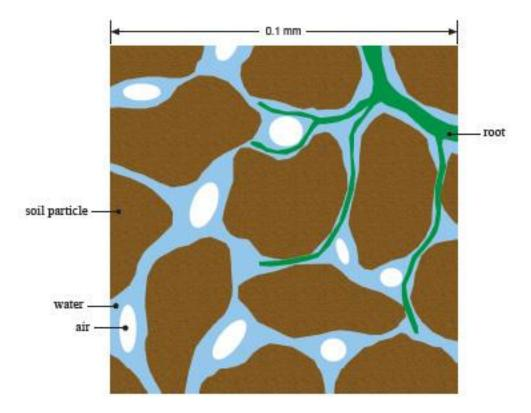
Figure G.1-3. Unsaturated Soil Composition
