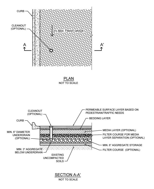
Typical Plan and Section View of a Permeable Pavement BMP
