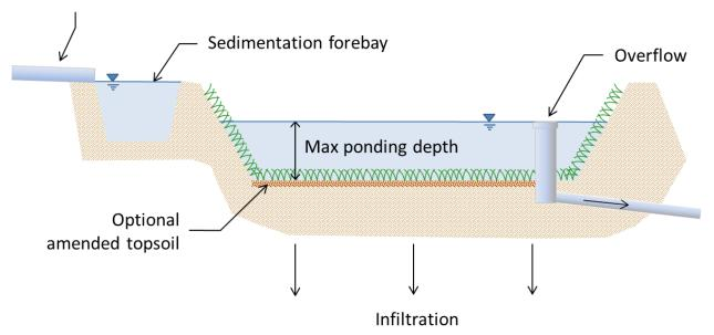
FIGURE 5-7. Schematic of a Typical Infiltration Basin
