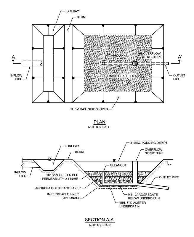
Typical Plan and Section View of a Sand Filter BMP
