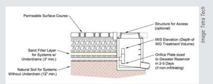
Figure 6-11. Permeable interlocking concrete pavement cross-section.
