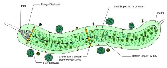
FIGURE 5-10. Schematic of a Vegetated Swale
