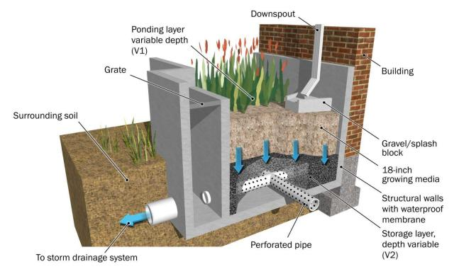
Biofiltration with impermeable liner BMP Example Illustration
