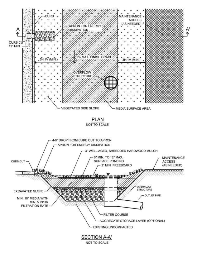
Typical Plan and Section View of a Bioretention BMP
