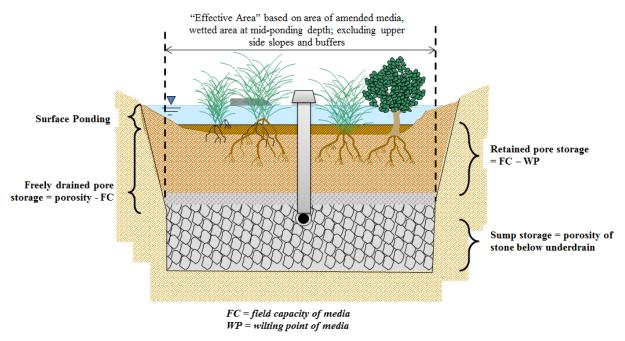
**Explanation of Biofiltration Volume Compartments for Sizing Purposes**
