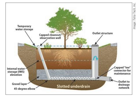
**Figure 4-25.** In this underdrain design cross-section image, an upturned pipe connected to a slotted underdrain ensures that a permanent internal water storage layer is maintained within the practice before the excess infiltrated water spills into a secondary drainage network. In this design, a surface overflow drain is included to provide added protection against high volume flows.
