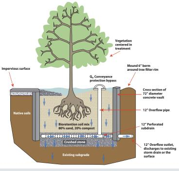
Figure 6-6. Stormwater tree pit schematic.
