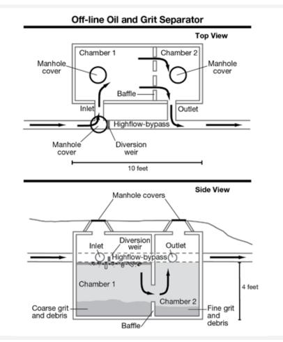
**Figure 5-3.** An off-line oil and grit separator diverts incoming stormwater into two chambers that slow flow and allow oil and grit to separate from the water stream.
