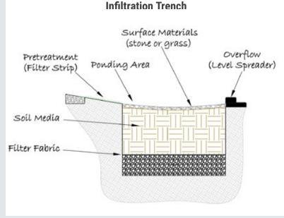
Figure 6-8. Stormwater infiltration trench schematic.
