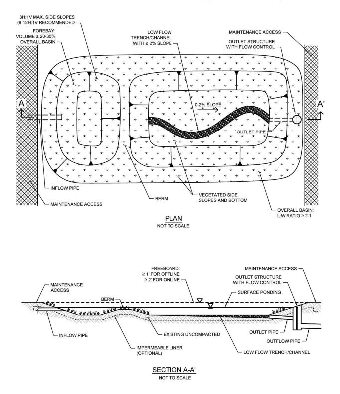
Typical Plan and Section View of a Dry Extended Detention Basin BMP
