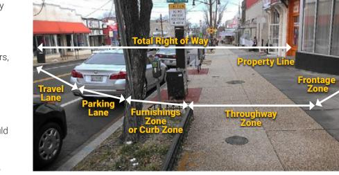
**Figure 2-5.** In this setting, pedestrian-friendly zones have a relatively high amount of space in the right-of-way relative to the size of the street.
