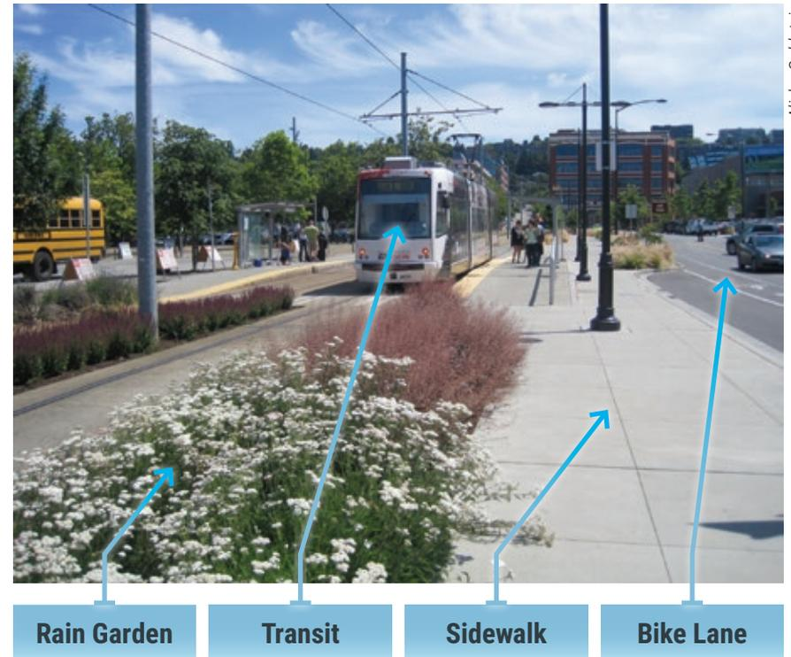
**Figure 1-4.** A green and “complete street” in Seattle, Washington, includes specific streetcar, vehicle, bike and pedestrian zones and a rain garden and vegetated stormwater curb extensions to capture and treat runoff.
