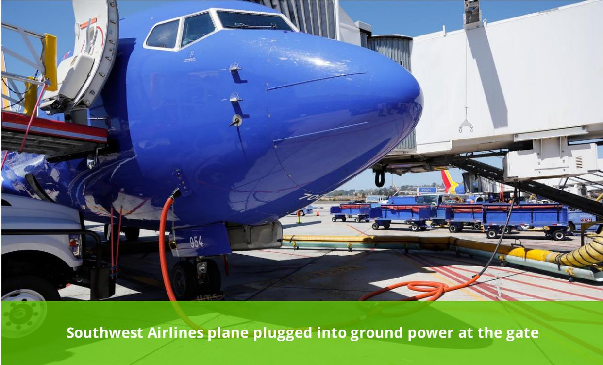
Southwest Airlines plane plugged into ground power at the gate
