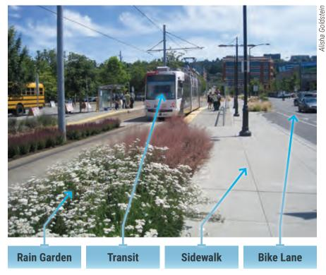
**Figure 1-4.** A green and "complete street" in Seattle, Washington, includes specific streetcar, vehicle, bike and pedestrian zones and a rain garden and vegetated stormwater curb extensions to capture and treat runoff.
