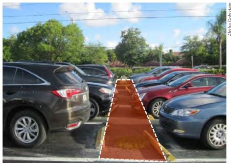
**Figure 2-13.** In this parking lot the impervious median space between facing parking stalls could be retrofitted to infiltrate runoff.
