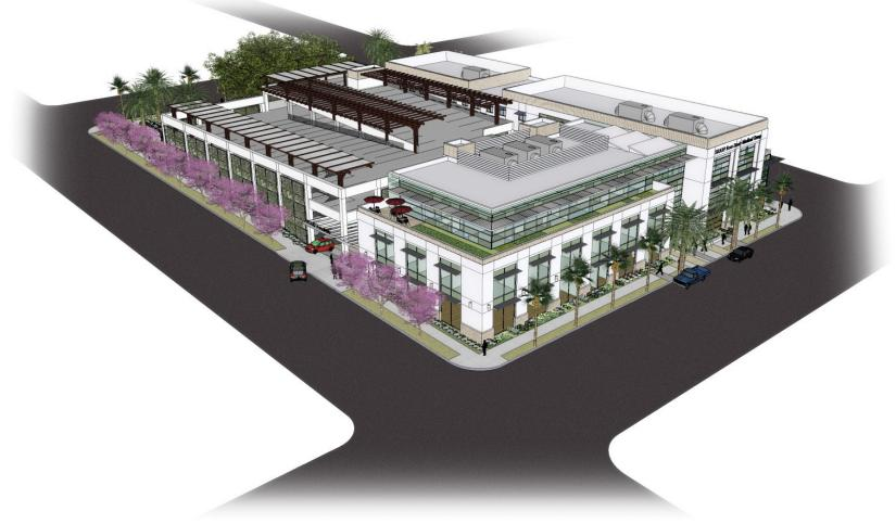
The building is designed to mitigate exterior noise, achieving an internal sound level of 45 dB. This meets the requirements of an avigation easement for any use.
