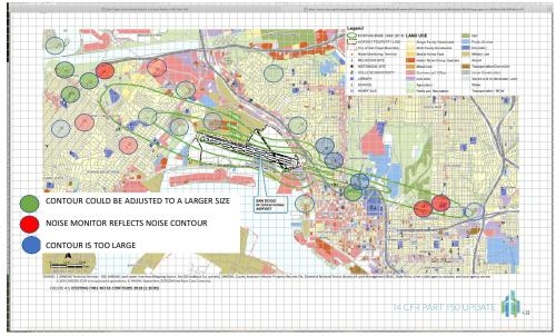
Figure 5 Part 150 2018 noise contour showing areas how noise monitors would adjust or refine the contour
