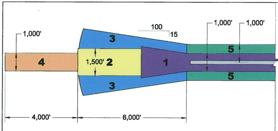
Note: As depicted, the dimensions of the Safety Zone 1 (Runway Protection Zone) are 1,000' x 1,750' x 2,500'; these dimensions may be adjusted based on each airport's approach types and approved RPZ dimensions.
