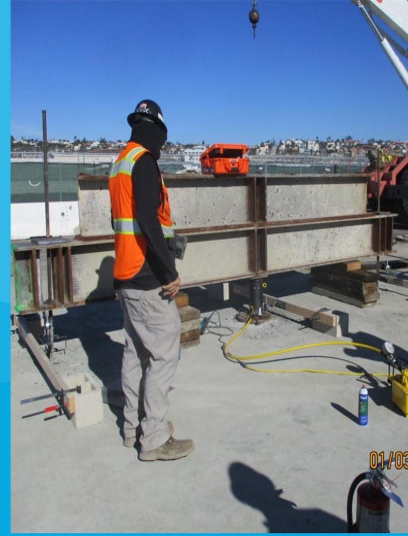
Stressing the Test Pile
