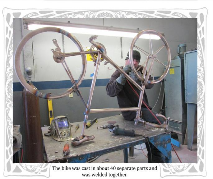
The bike was cast in about 40 separate parts and was welded together.
