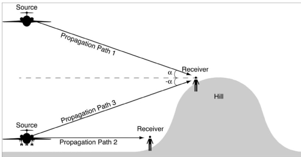
**Figure G-2 Aircraft Noise Propagation Paths to Receivers on a Hill**
