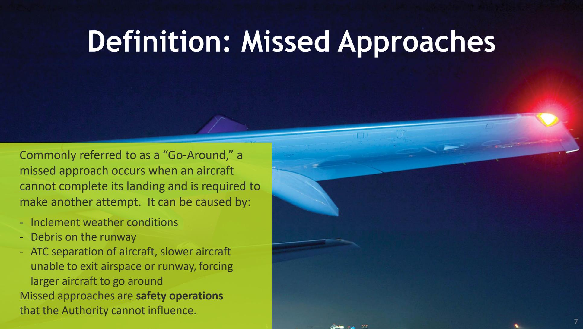
Commonly referred to as a “Go-Around,” a missed approach occurs when an aircraft cannot complete its landing and is required to make another attempt. It can be caused by:
