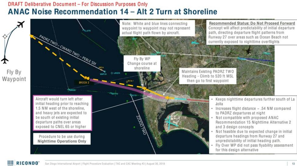
Figure 3 Nighttime alternative presented includes use of PADRZ SID for initial departure segment<sup>2</sup>
