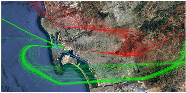
Aircraft at SAN typically operate in a "west flow" pattern where they arrive from the east and depart to the west. During inclement weather or high wind conditions they will operate in a reverse flow departing to the east and arriving to the west, however "east flow" is infrequent and represents approximately 1.7% of the total annual operations.
