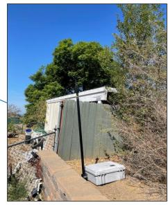
Figure 3. Portable Noise Monitor Set Up
