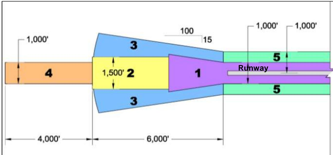
Caltrans recommends a standard safety zone configuration for large air carrier runways which may be adjusted to account for individual airport approach types and RPZ dimensions
