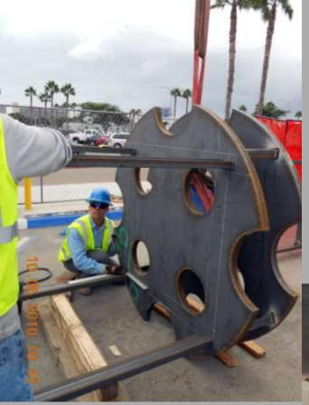
Test Caisson Load Cell
